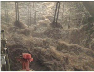
Example coarse bubble aeration, partly to keep membranes clean
